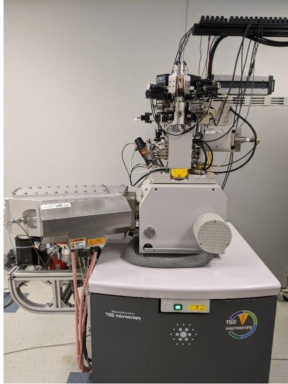
Figure 1: SIMS:ZERO system equipped with a cesium low temperature ion source. This system is installed at zeroK NanoTech.
