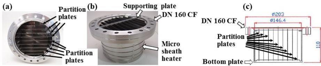
Fig 1. (a) A top view, (b) a side view from obliquely above, and (c) a sectional view of the vacuum vessel for the NEG pump before oxygen-free Pd/Ti deposition [1].
