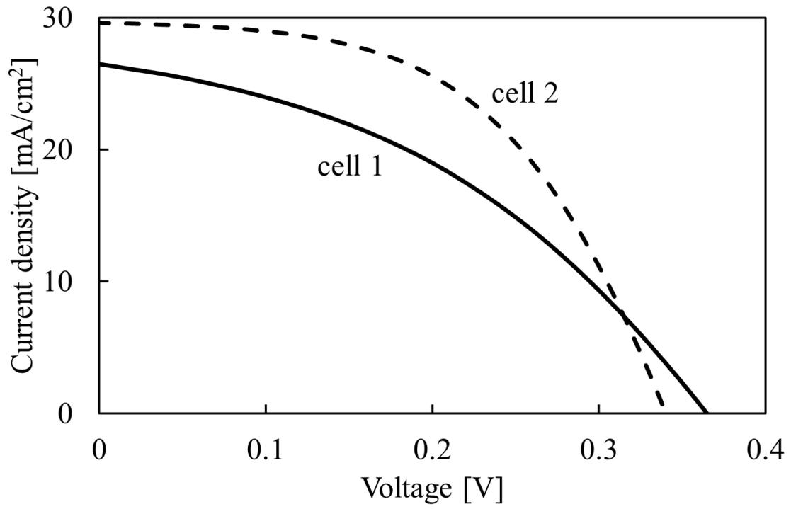
Figure 1.  $J$ - $V$  characteristics of cells 1 and 2.
