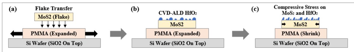
[Figure 1] Overall Process Procedure for Strain: (a) Flake Transfer at 100°C (b) CVD-ALD HfO 2 Deposition at 250°C (c) After Cooling at Room Temperature (25°C)
