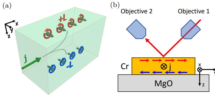
Figure 2. (a) Schematics of the orbital Hall effect. The charge current  $j$  generates a transverse orbital current, leading to orbital accumulation on the sample's surfaces. (b) Measurement setup utilizing the longitudinal MOKE to detect the in-plane orbital accumulation.
