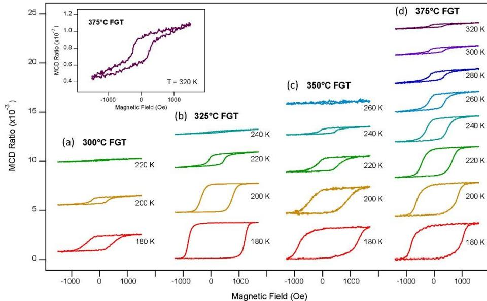
Figure 1. Temperature dependence of MCD loops for FGT samples ( $\sim 4$  nm) grown at  $300^\circ\text{C}$ ,  $325^\circ\text{C}$ ,  $350^\circ\text{C}$ , and  $375^\circ\text{C}$  on  $\text{Bi}_2\text{Te}_3$ .
