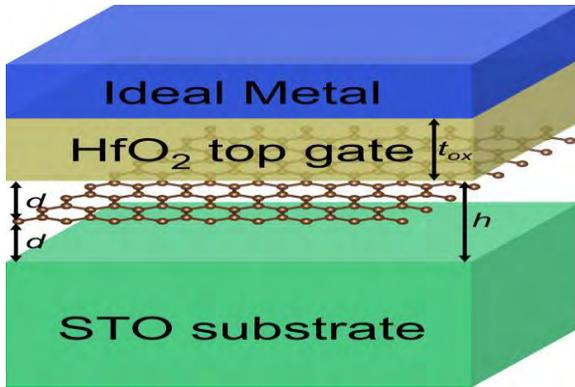
Figure 1. Schematic of a model used in our calculation. Here the STO substrate is assumed to be semi-infinite and the graphene layer is laterally infinite in the vacuum region between HfO<sub>2</sub> and STO.
