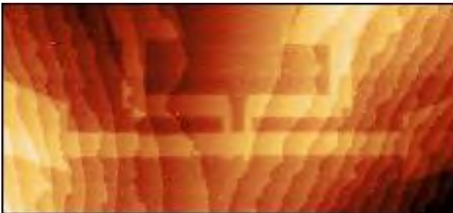
Figure 1 Lithographically defined device on Si(100) 2×1:H
