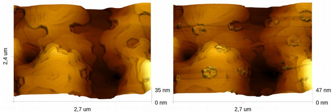
Figure 2. AFM topography image before (left) and after (right) applying 6 V sample bias
