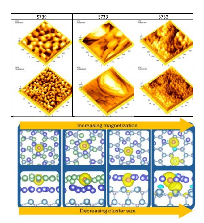
In the AFM image, it can be observed that sample S739 (which does not contain Mn) has not formed well-defined structures, whereas the sizes of these structures are clearly visible in samples S733 and S732. It is evident that the nanostructures in sample S732 are significantly smaller. The results of the DFT calculations are shown in the figure below, indicating that magnetization increases as the nanostructure size decreases.
