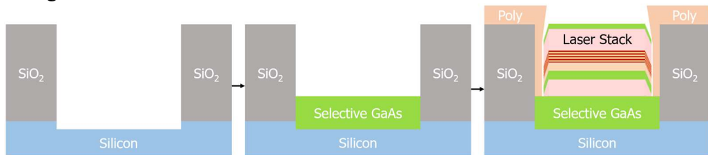
Figure 2: Illustration of the growth process of the quantum dot laser stack. A thick GaAs buffer is grown selectively in a pocket etched in a photonic integrated circuit chip. The lower cladding, active region, and upper cladding of the laser stack are then grown under conventional growth conditions.
