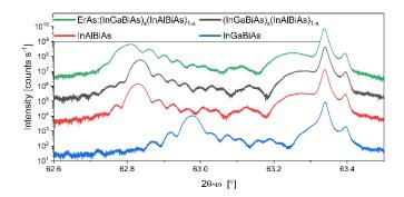
**3.** High-resolution X-ray diffraction (004)  $2\theta - \omega$  coupled scans of 300 nm strained [ErAs:(InGaBiAs)x (InAlBiAs)1–x] films with  $\sim 3.5\%$  Bi and  $\sim 1\%$  ErAs.
