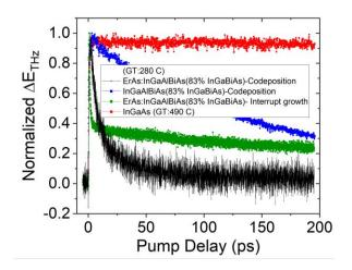
Carrier dynamics measurement by Optical pump THz probe spectroscopy GT= Growth Temperature.
