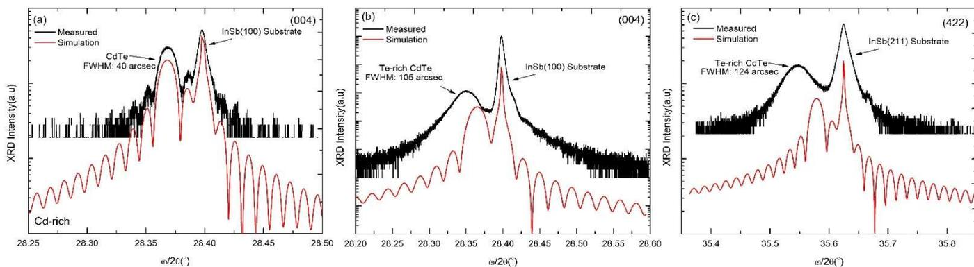
Fig. 1. XRD spectra of CdTe grown under (a) Cd-rich conditions on InSb(100) substrate, (b) Te-rich conditions on InSb(100) substrate and (c) Te-rich conditions on InSb(211) substrate. CdTe layers grown under Cd-rich conditions result in high-quality films while Te-rich conditions have an increased linewidth and shifted peak position indicating alloying.
