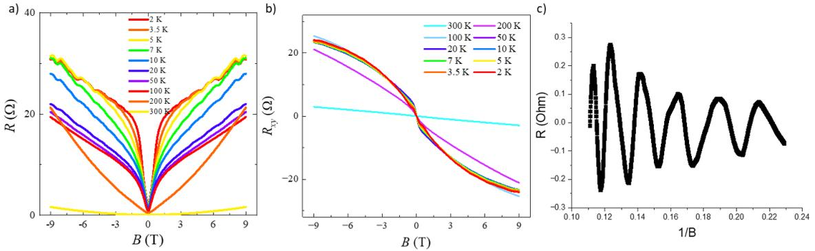
Fig. 2.  $\alpha$ -Sn and dilute Ge alloys exhibit large magnetoresistance, Shubnikov-de Haas oscillations and weak antilocalization (a,b). Expanded Shubnikov-de Haas quantum oscillations as a function of inverse magnetic field (c).
