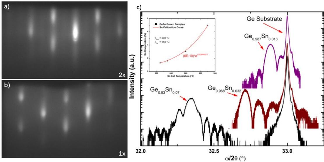
Fig. 3. RHEED reconstruction changes from ( $2 \times$ ) to ( $1 \times$ ) with increasing Sn composition (a,b). XRD spectra of GeSn samples towards achieving  $k$ -SCS with increasing Sn content, showing nice Pendellösung fringes (c). (inset) Sn composition versus Sn cell temperature calibration curve for constant substrate and Ge cell temperature.
