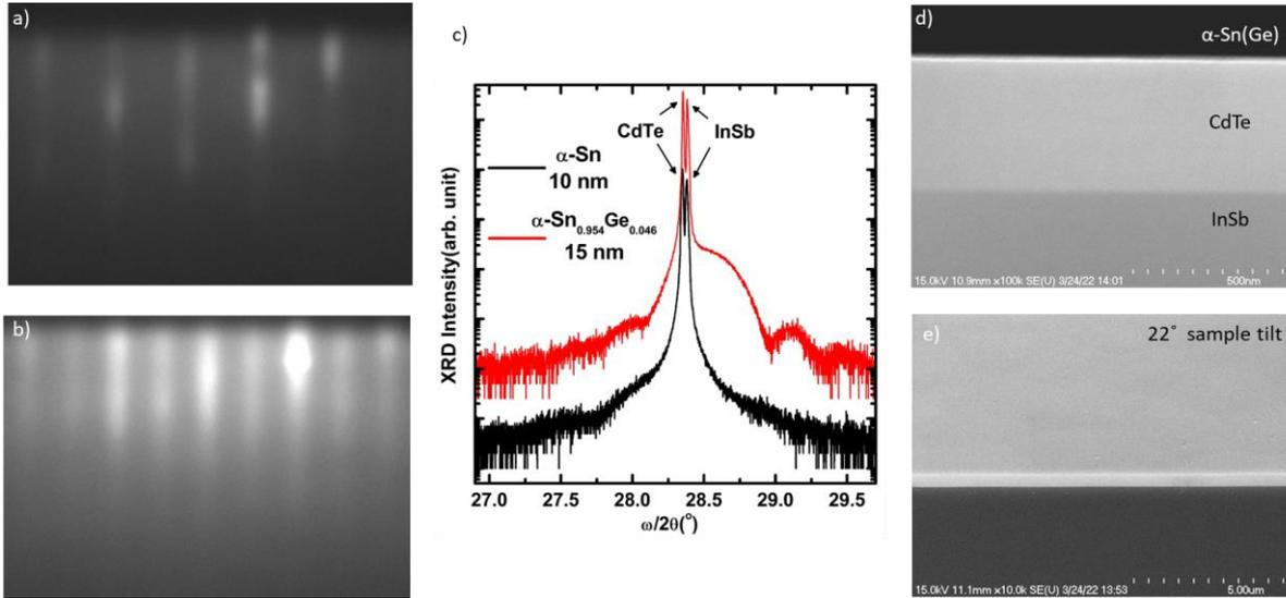
Fig. 1. After a few monolayers of  $\alpha$ -Sn(Ge) growth, RHEED becomes a streaky ( $2 \times 2$ ) pattern (a,b). The thickness and Ge composition were determined from XRD simulation and Pendellösung fringes (c). Cross sectional SEM imaging confirmed thickness and showed single crystal layers with abrupt interfaces between  $\alpha$ -Sn(Ge)/CdTe/InSb (d) and smooth surfaces (e).
