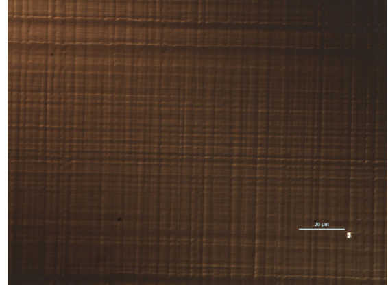
Nomarski microscopy images of InGaSb graded buffers grown at T_{\text{sub}}=455\text{ }^{\circ}\text{C} (left) and 495\text{ }^{\circ}\text{C} (right)
