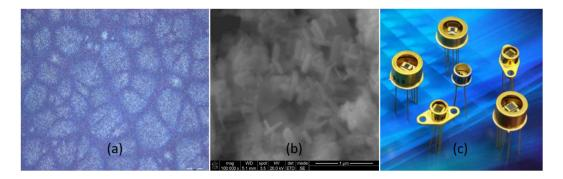
Figure 1(a) shows a micrograph of the snowflakes patterns, while Figure 1(b) shows the formed nanoprisms entangled with each other, which were revealed after etching the oxide phases of the PbSe matrix. Examples of PbSe detectors (www.optodiode.com) fabricated based on such nanostructures are shown in Figure 1(c). It is clear that underneath the snowflakes patterns, many nanoprisms are developed, massively entangled together, and form clusters of nanostructures.
