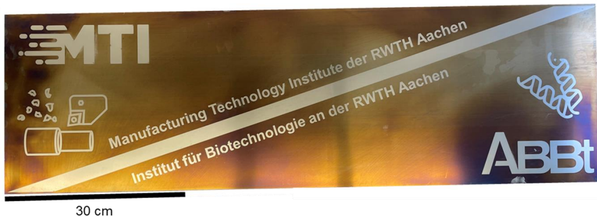
Figure 2: Validation of the scalability of the enzymatic coating method by coating a stainless-steel plate measuring 30 × 100 × 0.02 cm.
