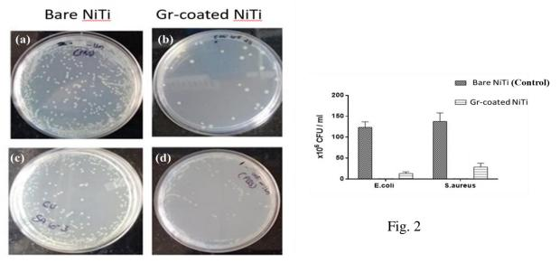
Fig. 1 shows digital image of petriplates of bare Nitinol substrate (a,c) and graphene-coated samples (b,d) for E.Coli bacteria (a,b) and S.Aureus (c,d). Fig.2 shows cell-viability assay for both bare and graphene-coated samples.
