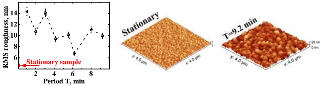
Figure 1: Left: Evolution of the rugosity as a function of the Oscillation Period T. Right: AFM of a coupled selected samples.
