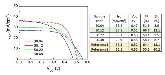
J-V curves and device efficiency of measured in samples with various S/(S+Se) ratios, the highest cell efficiency obtained in this study was 12.1%, this degree of efficiency is close to that of the reference specimens using toxic  $H_2Se/H_2S$  gases
