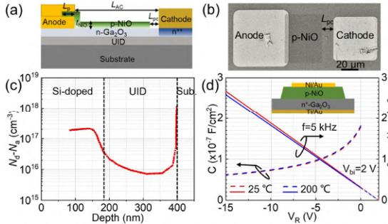
Fig. 1. (a) Schematic diagram and (b) top-view SEM image of the RESURF Ga<sub>2</sub>O<sub>3</sub> SBD. (c) The  $N_d-N_a$  depth profile of the Ga<sub>2</sub>O<sub>3</sub> epi layers. (d) C-V and  $1/C^2$ -V characteristics of the vertical NiO/Ga<sub>2</sub>O<sub>3</sub> diode at 25°C and 200°C.
