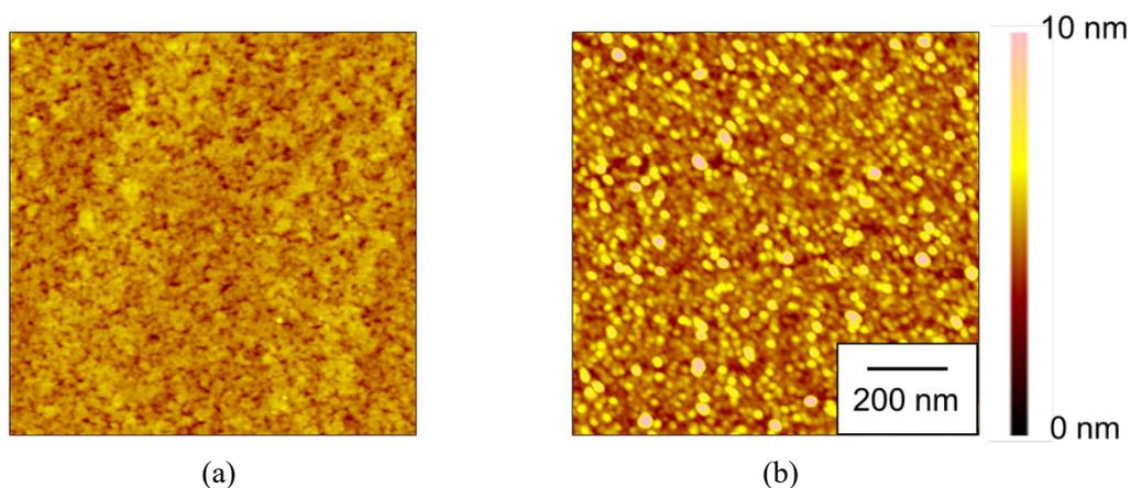
Fig. 1 AFM images of  $\text{Ga}_2\text{O}_3$  (a) (100) and (b) (010) surfaces after 120-min N radical irradiation.
