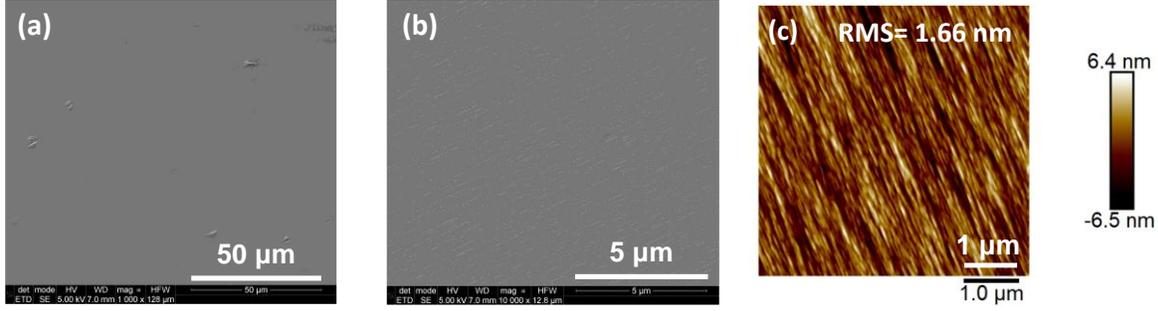
**Figure 1.** Top view FESEM images of MOCVD grown (010)  $\beta$ -Ga<sub>2</sub>O<sub>3</sub> thin film with growth rate of 3  $\mu\text{m/hr}$  and room temperature mobility of 190  $\text{cm}^2/\text{Vs}$ : (a) large field of view; and (b) high magnification. (c) The corresponding AFM image of the same  $\beta$ -Ga<sub>2</sub>O<sub>3</sub> sample (RMS: 1.66 nm).
