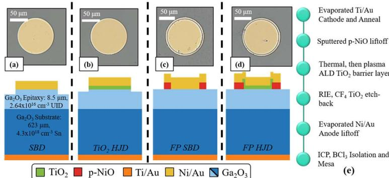
**Fig. 1** Optical microscope and cross section graphic depicting each device type: (a) SBD (b) TiO<sub>2</sub> HJD (c) GR SBD (d) GR HJD; and (e) an outline of the fabrication process flow.
