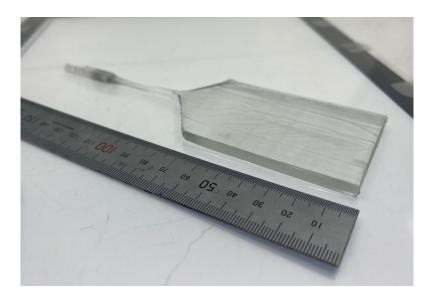
The typical bulk  $\beta$ -Ga<sub>2</sub>O<sub>3</sub> single crystal ribbon grown by EFG method. The growth direction and the principal surface were set to be the [010] direction and the (001) plane for this  $\beta$ -Ga<sub>2</sub>O<sub>3</sub> crystal, respectively. The ingot's body height and thickness are about 80mm and 4mm, respectively. The growth rate for this ingot is about 15mm/h.
