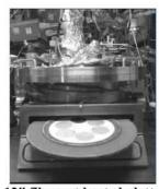
12" filament heated platter Platter (6 × 2") moving out from reactor
