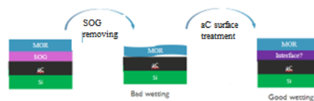
Figure 1 An approach to remove the SOG from the standard flow in order to have a good adhesion between MOR and aC
