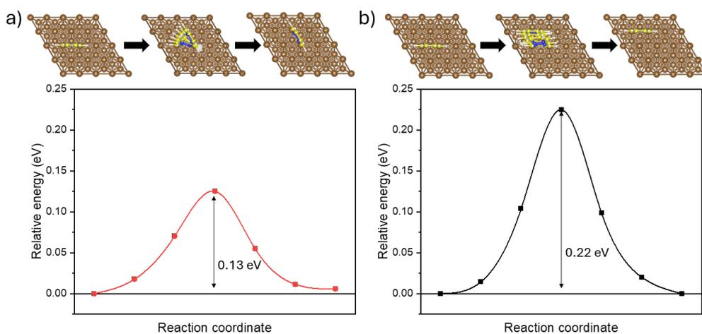
**Figure 3:** a) Rotation and b) diffusion of pyridazine on Cu (111) surface
