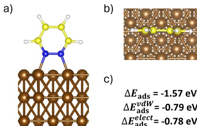
**Figure 1:** a) side, and b) top view representations of optimized pyridazine molecule on Cu (111) surface. c) total adsorption energy of pyridazine on Cu(111) surface and its electronic and dispersion components.
