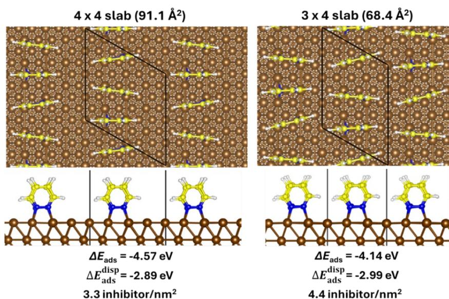
**Figure 2:** Top and side views of 4 x 4 and 3 x 4 supercells of Cu (111) surface saturated with pyridazine molecules. In ideal case, pyridazine molecules can favorably adsorb on Cu surface up to 4.4 molecules per nm<sup>2</sup>. In real conditions, it is expected to observe a surface saturation density between RSA and DFT calculated values.
