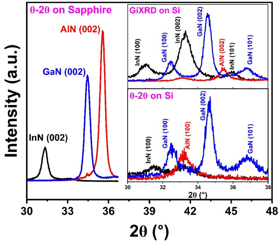
Figure 1. XRD and GIXRD scans of AlN, GaN, and InN on Si and Sapphire substrates
