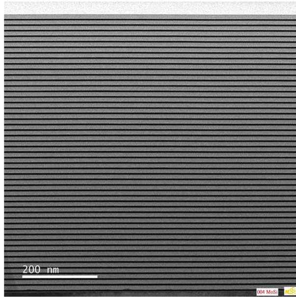
Fig. 1. Cross-sectional TEM image of the periodic Mo/Si bilayers by sputtering using cooling system.
