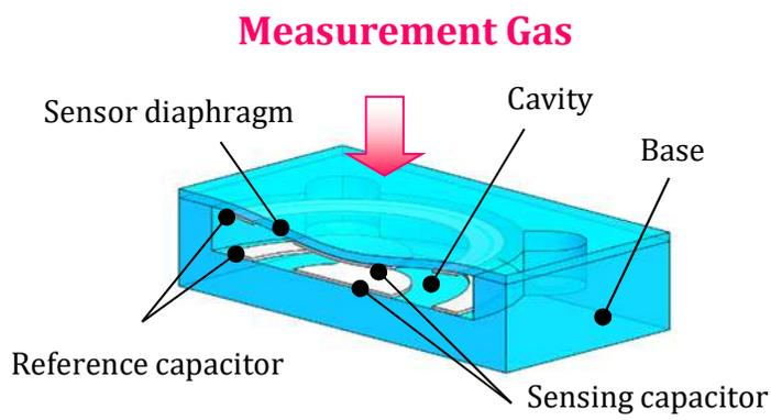
**Fig.1 Schematic cross-sectional view of sapphire-based capacitive pressure sensor chip**
