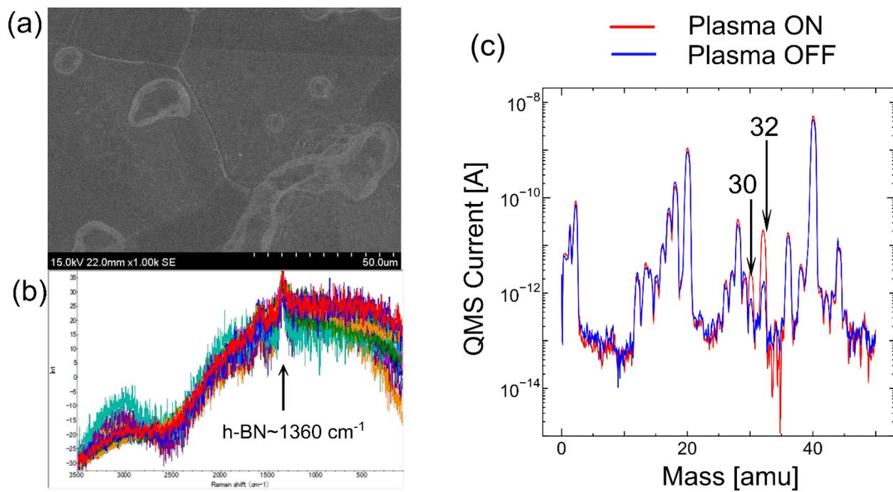
Figure 1. (a) SEM image of h-BN thin film grown on copper substrate. (b) Raman spectrum of grown h-BN thin film. (c) Difference in mass spectra downstream of Ar-diluted ammonia borane plasma with and without plasma.
