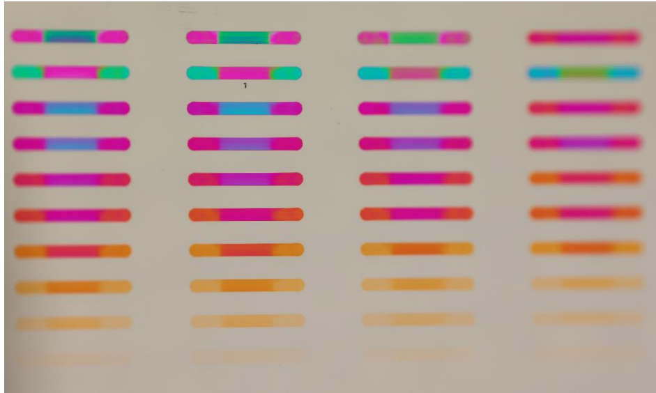
Figure 1. Photograph of a set of \text{TiO}_2 lines deposited using \mu\text{DALP}^{\text{TM}} at differing numbers of cycles (ranging from 100-5000) on a 200 nm \text{SiO}_2 substrate. \text{TiO}_2 was deposited using TTiP and water.
