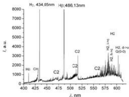
Figure 3. Typical spectrum of reversed arc discharge in Ar+H<sub>2</sub>+CH<sub>4</sub> gas mixture at RA current of 144A.
