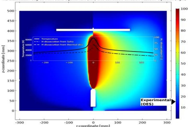
Figure 4. Comparison of the modeling distributions of H<sub>2</sub> dissociation degree across the column of 10%Ar-90%H<sub>2</sub> arc at  $p=2$  mTorr and  $I=150$ .
