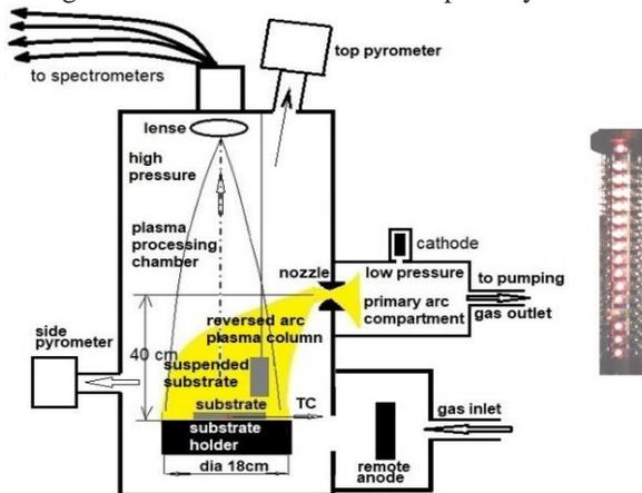
Figure 1. Schematic diagram of a reversed arc discharge reactor with stationary substrate (left); and photograph of the 1 meter tall, fluidized bed reactor tube for diamond growth on in-flight aerosol particles in operation (right).
