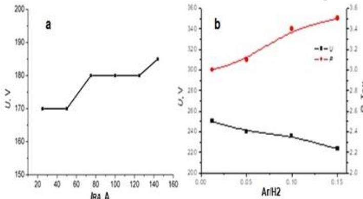
Figure 2. RA discharge voltage as functions of RA current at P=2 Torr and Ar/H<sub>2</sub>=0.14 (a); discharge voltage and gas pressure in the plasma processing chamber as functions of Ar/H<sub>2</sub> ratio at P=2 Torr and I=144A (c).
