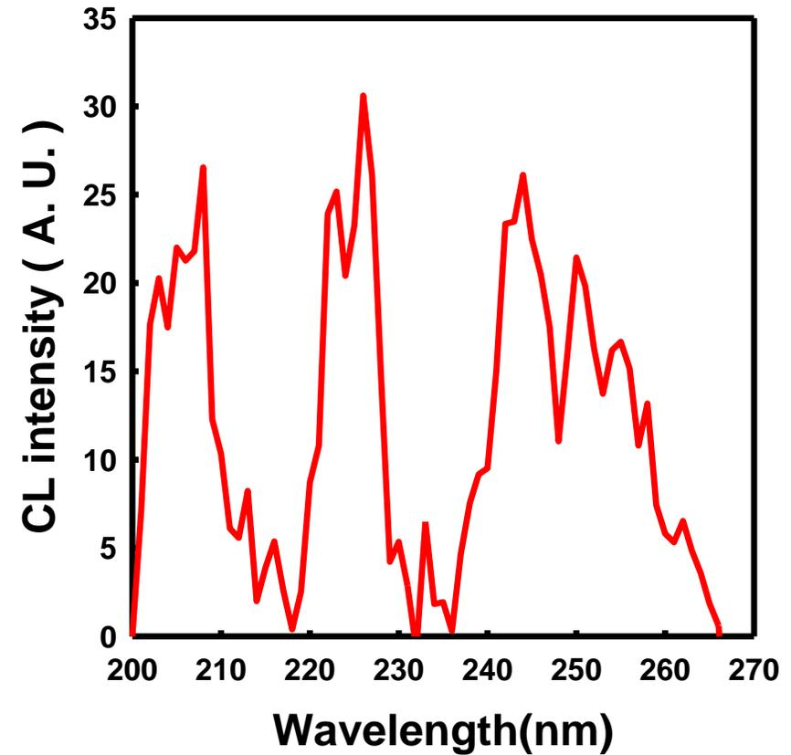
Emission peak of UV light with CNT based cold cathode electron beam. Peak position depend on the anode layer fabrication process.
