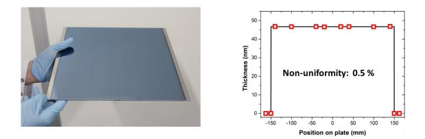
Fig. 1: Left: Photograph of a 325 mm x 325 mm aluminum covered glass plate with 90 nm Al<sub>2</sub>O<sub>3</sub> deposited by large area spatial ALD. The blue color is caused by interference and is used to visualize the thickness uniformity. Right: the film thickness measured by ellipsometry, showing non-uniformities < 1%.</p>
