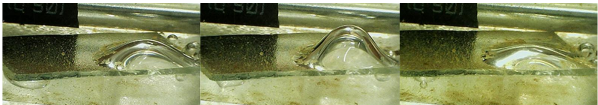
Figure 2 – Plastron regeneration in seawater illustrating a sustained plastron evident by the reflective surface on the substrate.
