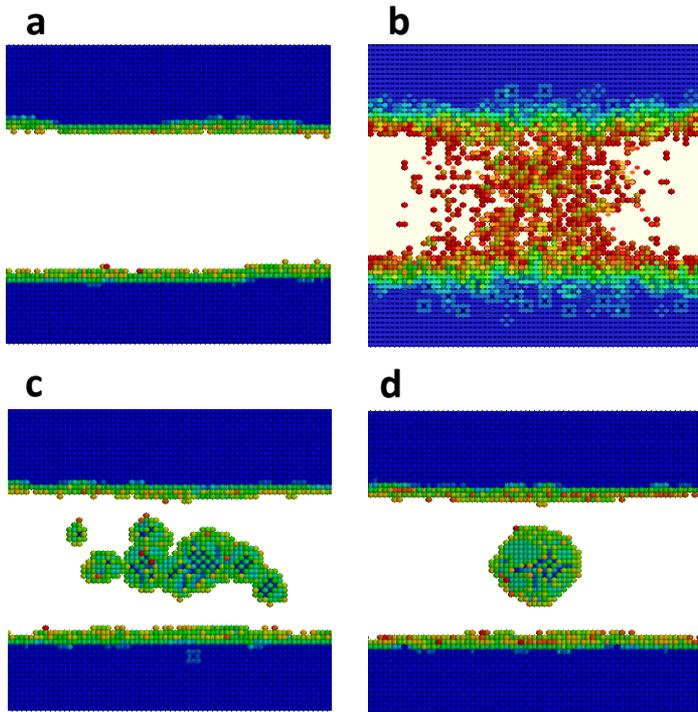
**Figure 1.** (up) TRIDYN and 3DkMC simulation shows formation of a single Si ND via (a)(b) ion beam mixing and (c)(d)thermal treatment.
