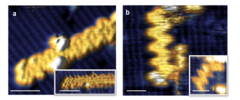
Figure a. High resolution STM images of double-wide GNRs on InAs (110) with the As <u>sublattice</u> clearly seen; inset shows the hexagonal superstructure of the GNR (scale bars are 3nm).
