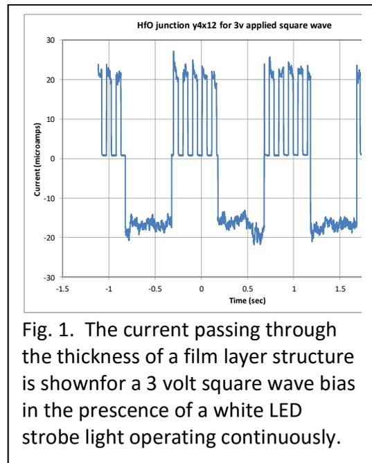
Fig. 1. The current passing through the thickness of a film layer structure is shown for a 3 volt square wave bias in the presence of a white LED strobe light operating continuously.
