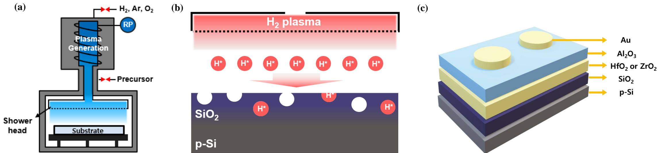
Fig 1. Schematic Diagrams of (a) the ALD and HPT in-situ process chamber, (b) HPT effect, and (c) CTM devices studied in this study.
