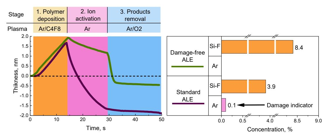
**Figure 1.** One cycle of PEALE SiO2. 1. Polymer deposition in down-stream ICP mode similar to PEALD. 2. Activation of surface reactions by low-energy ions in damage-free PEALE. Products removal in standard PEALE. 3. Products removal and chamber cleaning by oxygen atoms reactions.
