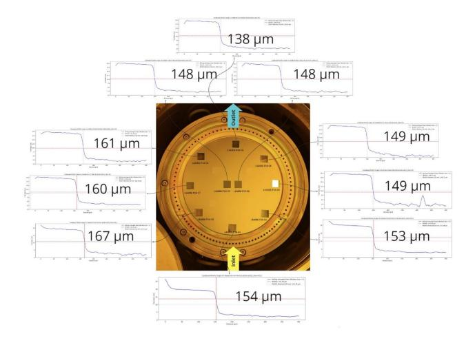
**Figure 1.** Conformality data obtained with a 200 mm PillarHall pocket wafer. The penetration depth measured using a thin film analyzer reflectometer (Filmetrics F40-UVX) is given.
