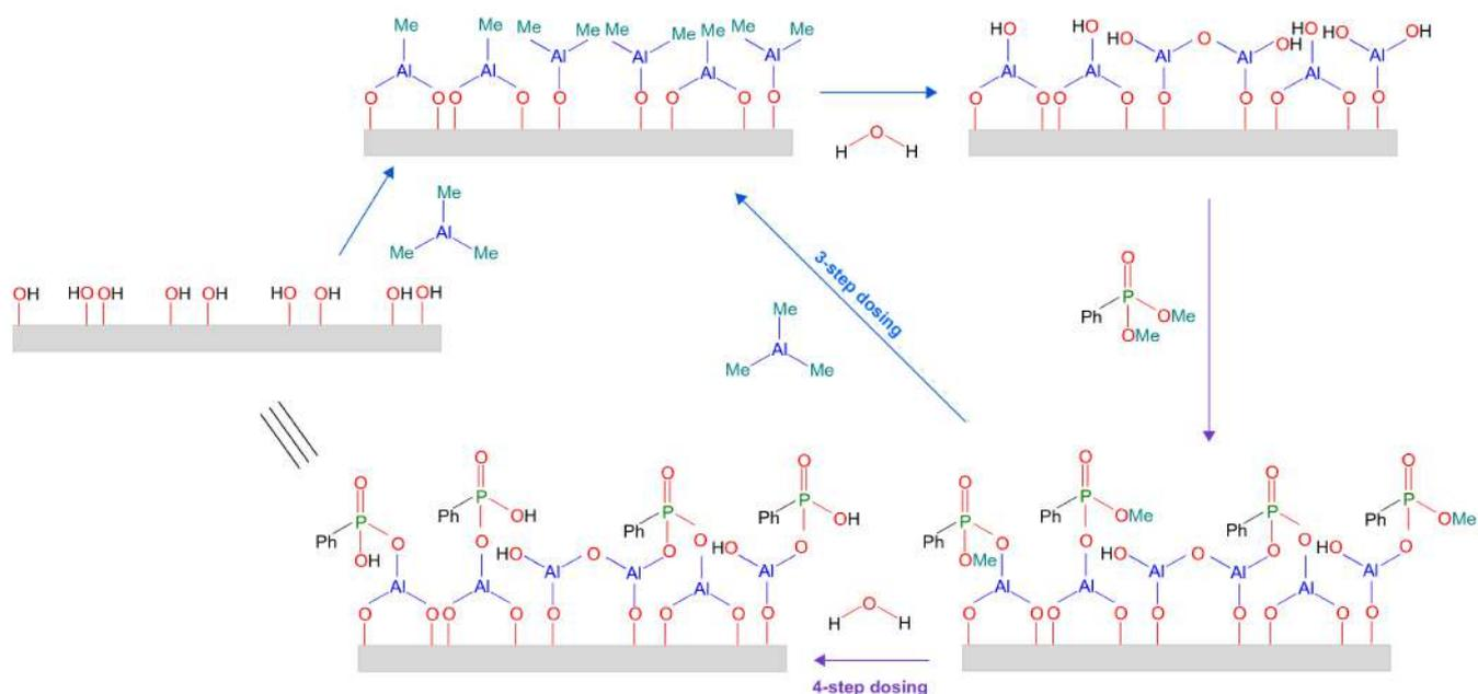
Figure 1: Schematic representation of the different dosing sequences used for the deposition of aluminium phenylphosphonate (AlPhPO) films based on our proposed reaction chemistry.
