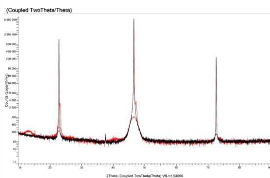
Figure 2. X-ray diffractogram of  $\text{NdFeO}_3$  thin film on  $\text{SrTiO}_3(001)$  as deposited (black) and after annealing (red).
