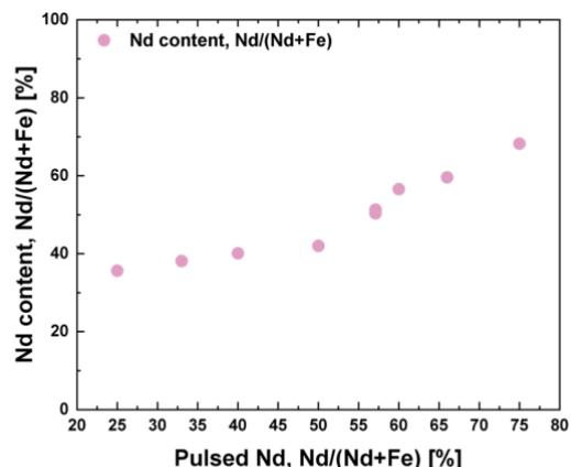
Figure 1. Neodymium content (atomic %) in  $\text{NdFeO}_3$  thin films deposited on Si-substrates as a function of amount of Nd pulsed (atomic %).
