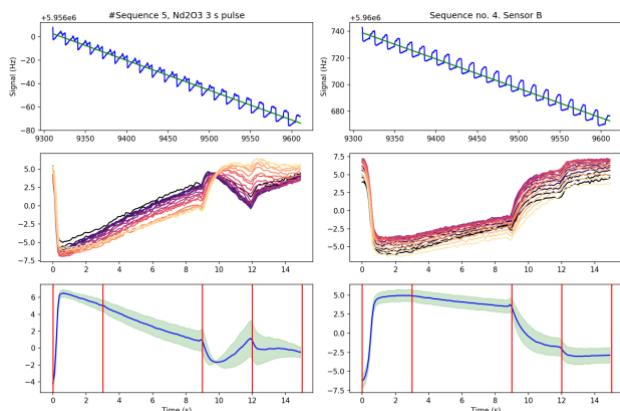
Figure 3. Excerpt of quartz crystal microbalance measurement during a deposition of  $\text{NdFeO}_3$  thin films, showing frequency change for a 3 s long Nd pulse.
