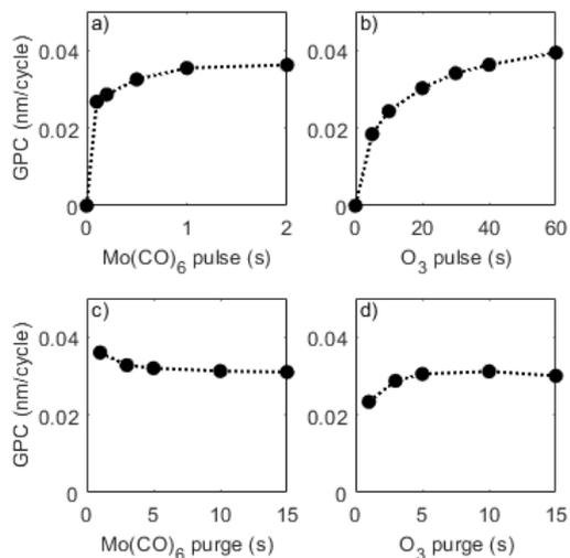
Figure 1 –GPC as a function of a)  $\text{Mo(CO)}_6$  pulse time, b)  $\text{O}_3$  pulse time, c)  $\text{Mo(CO)}_6$  purge time, and d)  $\text{O}_3$  purge time, as determined by in-situ spectroscopic ellipsometry (SE).
