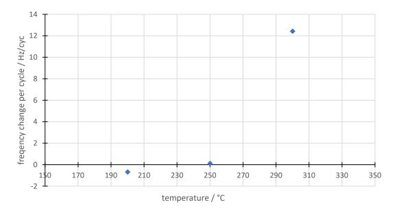
Dependence of the frequency change per cycle on the process temperature at 10 s precursor pulse time, with layer deposition at 200 °C, limited range between deposition and etching at 250 °C and pulse time-dependent etching at 300 °C
