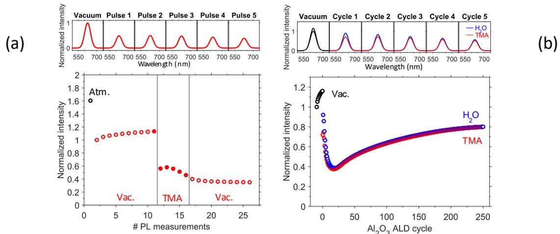
Fig. 1. Evolution of the integrated QD photoluminescence with exposure to (a) 5 pulses of trimethylaluminum (TMA) and (b) 250 cycles of  $\text{Al}_2\text{O}_3$  ALD.
