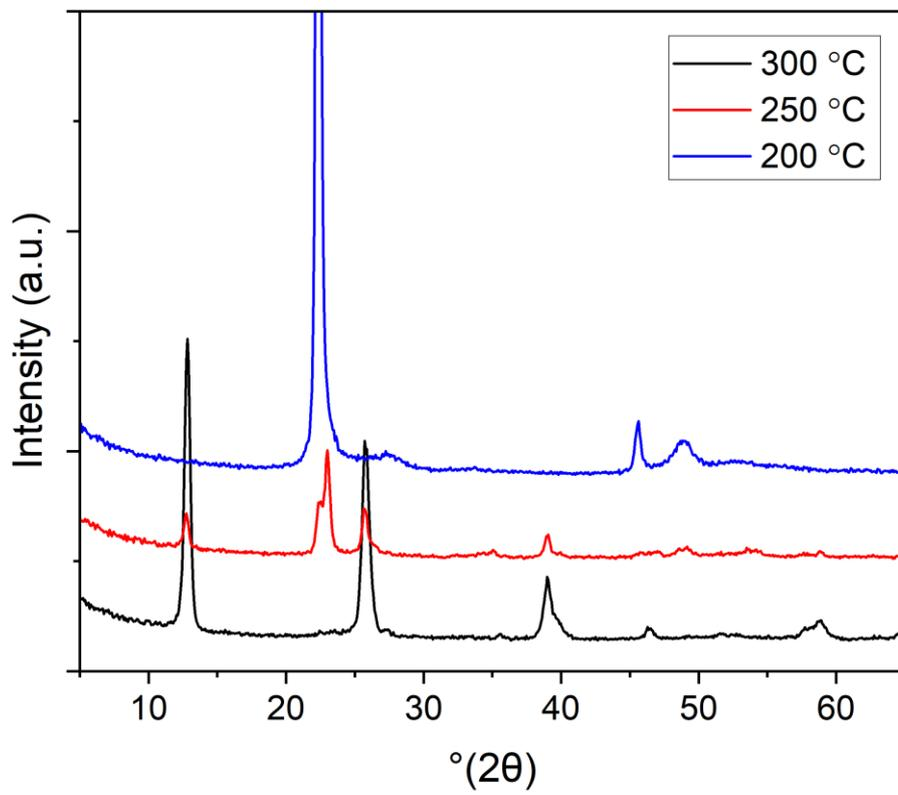
Figure 2. XRD diffractograms of MoO<sub>x</sub> films deposited at different temperatures.
