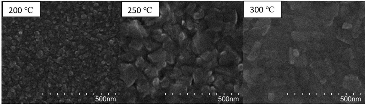
Figure 1. SEM images of MoO<sub>x</sub> thin films deposited at various temperatures.
