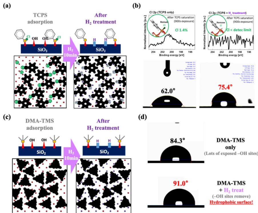
Fig. 2. (a) The hydrogen treatment mechanism and changes in surface condition, and (b) Cl 2p XPS peak and increased WCA diagram of the surface before and after hydrogen treatment for the TCPS adsorption surface. (c) The hydrogen treatment mechanism and changes in surface condition, and (d) increased WCA diagram before and after hydrogen treatment for the DMA-TMS adsorption surface.
