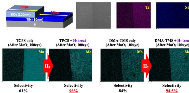
Fig. 3. AES element mapping (Ti, Si, and Mo) of SiO<sub>2</sub>/TiN patterned substrates after 100 cycles of AS-ALD MoO<sub>2</sub> using TCPS and DMA-TMS before and after applying hydrogen treatment.
