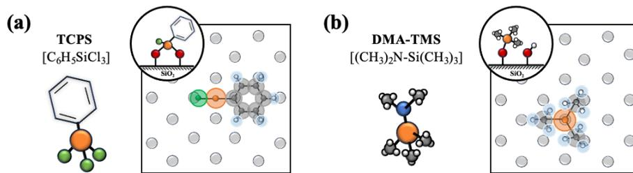
Fig. 1. The molecular structure, the form of the adsorbed SMI on the SiO<sub>2</sub> surface (top view), and the 2D footprint transcribed through Van der Waals area of (a) TCPS and (b) DMA-TMS.
